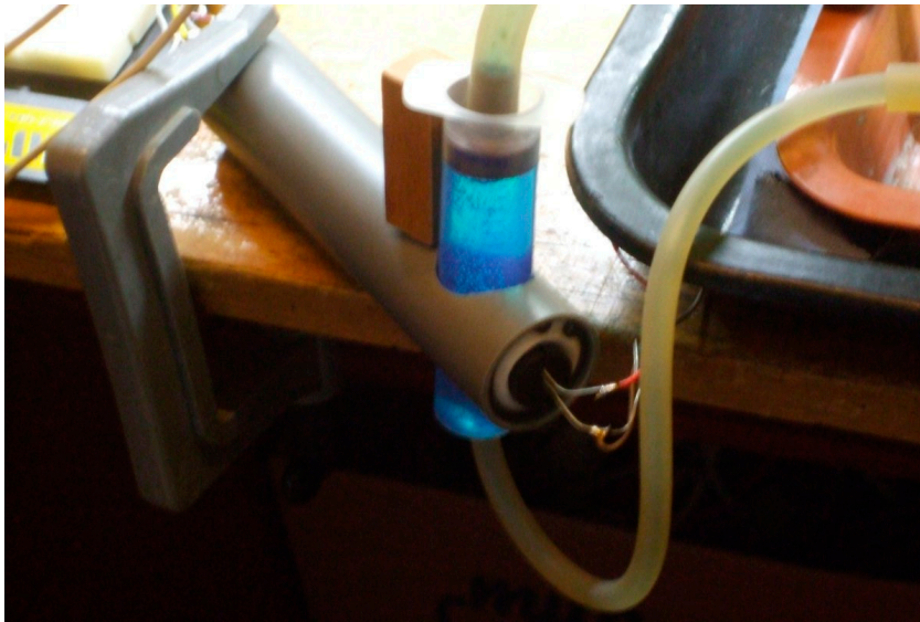
Figure 7. Detail of syringe (1) through which the intensity of the transmitted light is measured.
