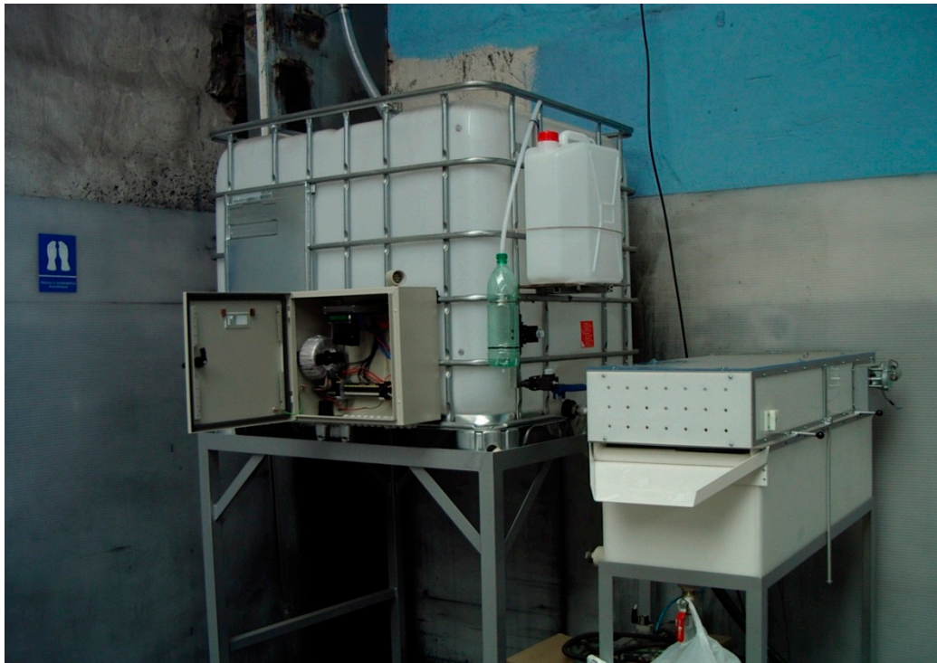
Figure 4. View on the equipment of the wastewater cleaner with the detail of the control box that is open.
