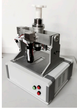
Figure 2. Prototype of the designed 3-DOF haptic master
