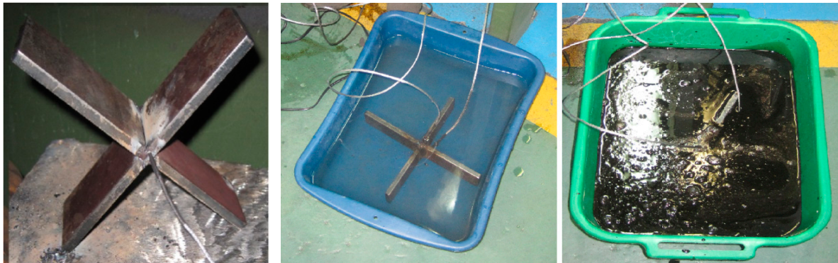
Figure 1. Connection of the thermocouples.
