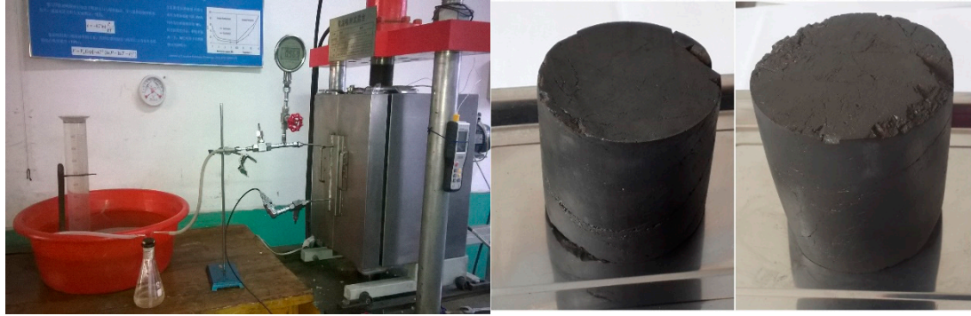
Fig.1 Experimental apparatus and coal samples used in these experiments (The left is experimental apparatus, the middle is Coal sample 1# and the right is coal sample 2#.)
