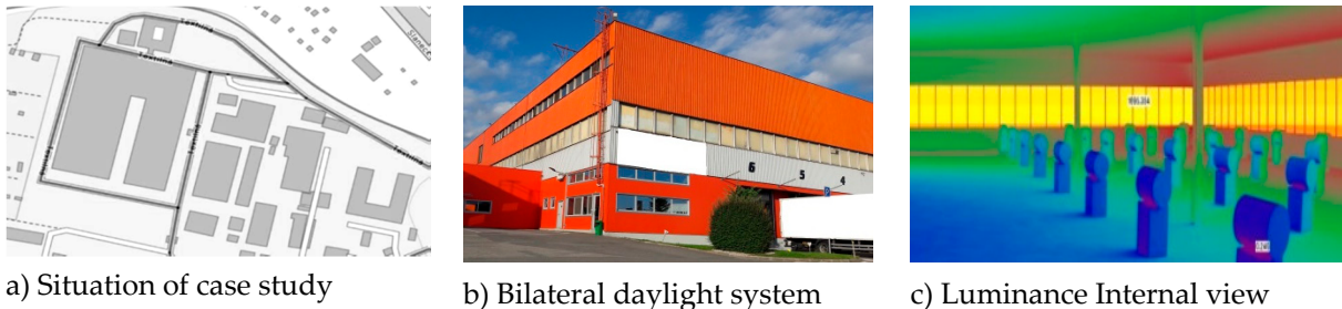
Figure 3. The situation of a textile factory placement, lighting simulation results near windows in double-side window day illumination
