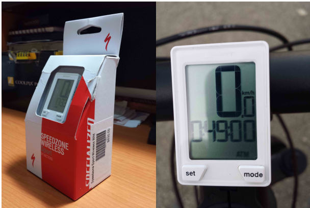
Figure 1. Cycle computer (Specialized Speed Zone Sport Wireless) receives data from a sensor mounted on the suspension fork.
