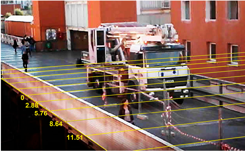
Figure 9: A frame of the camcorder video with the truck leaving the bridge. The transverse beams on the deck are used to obtain the position in the direction parallel to the longitudinal axis of the bridge.
