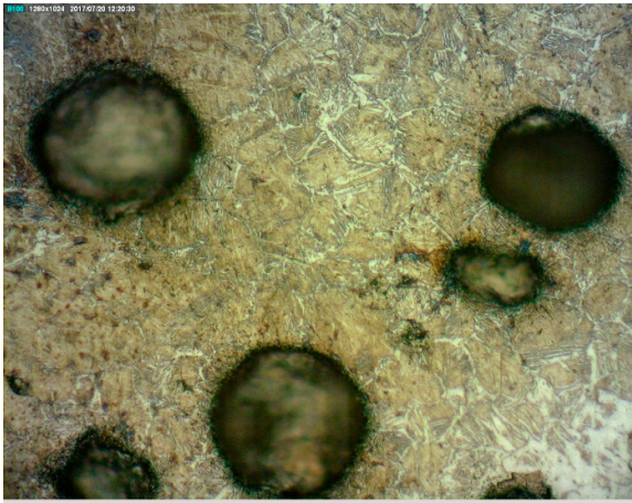
Figure 4.4. Austempered at 352°C with salt bath agitation, magnification 200x
