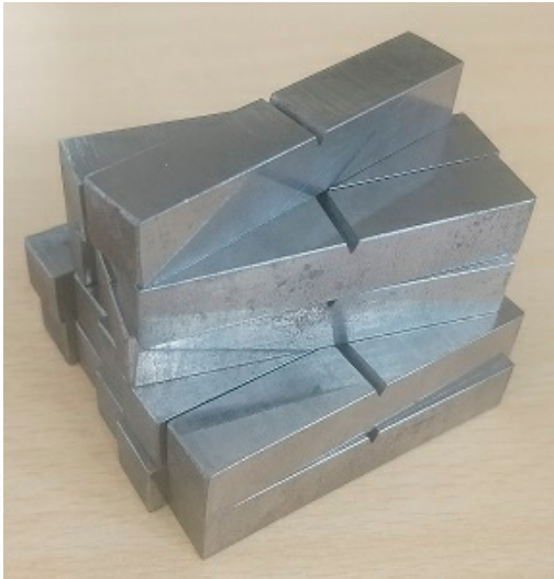
Figure 3.1. Standardized Charpy samples ready for experiments
