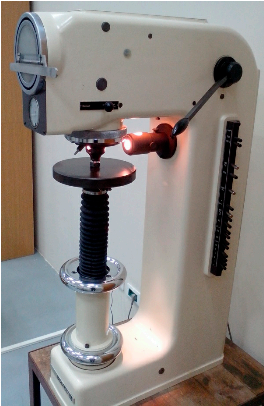
Figure 4.10. Wolpert hardness measuring machine
