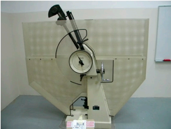
Figure 4.11. Wolpert Charpy pendulum
