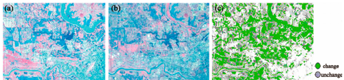
Figure 6. Remote sensing image for (a) 2000, (b) 2010 and change objects for a threshold of 0.72 similarity function (c).
