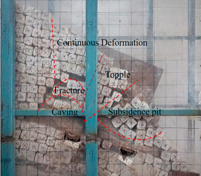
(c) Deformation of test model after mining #3 ore body
