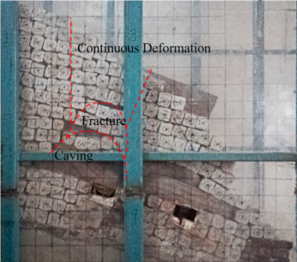
(c) Deformation of test model after mining #1 ore body
