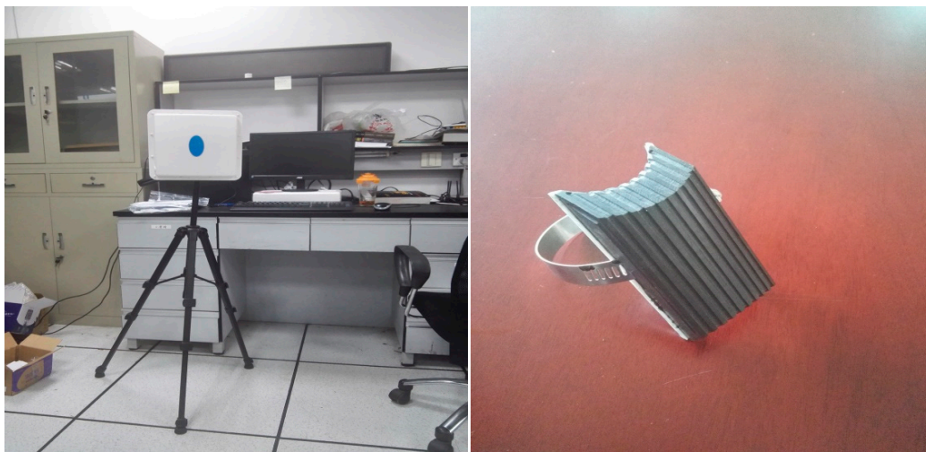
Figure 9. Indoor test environment, tag and reader. The tag is installed on the waist of pedestrian and the readers are mounted on tripods.
