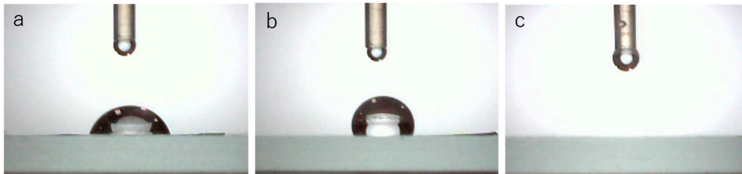
Figure 2 The shapes of the water drops applied to each sample.
