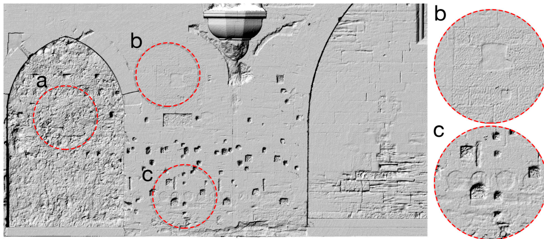
Figure 7. Raster Hillshade 315° azimuth 45°: (a) surface roughness not visible from photographs, (b) surface roughness not visible to the naked eye, and (c) carved symbols, barely visible on site.
