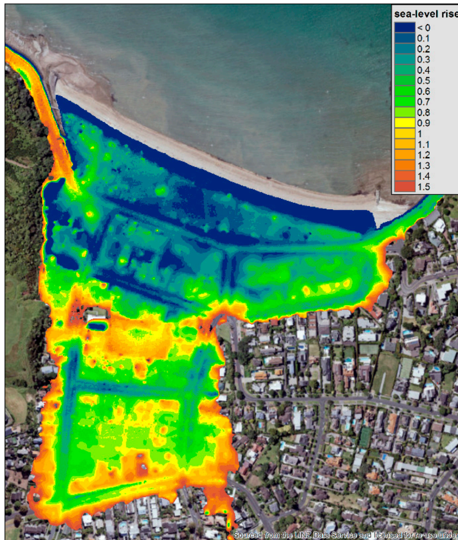
Figure 5. The effect of 0.1 m SLR increments on coastal-storm inundation exposure at Mission Bay (Auckland). SLR increments have been added onto the 1% AEP storm-tide elevation, which was calculated for the present-day mean sea level.
