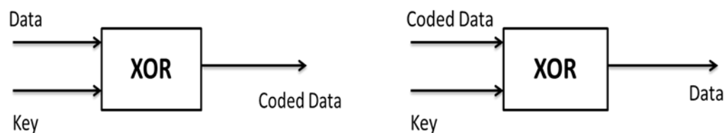
Figure 19 The left figure is the schematic of encryption. The right figure is the schematic of decryption. The same key stream is used for both encryption and decryption.
