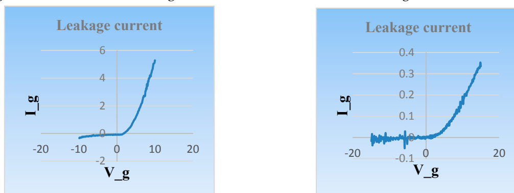
Figure 13. The gate leakage current of tow devices.
