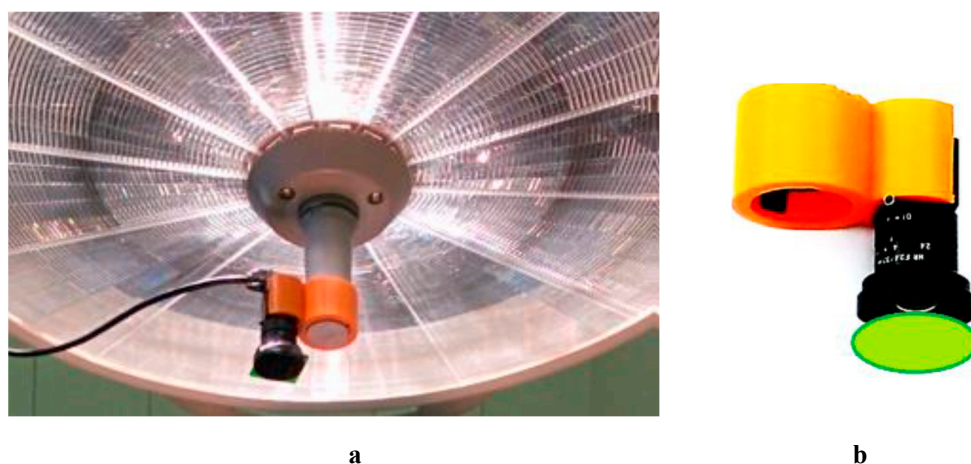
Figure 12. The PPGI device attached to a surgical lamp (a) and the design of its holder (b) [47].
