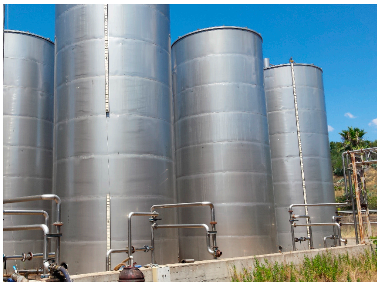
Figure 3. Silos stocking the olive juice obtained in Sicily in 2016 from a two-phase olive mill.
