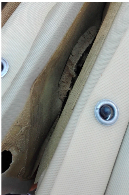
Figure 2. Solid-cake resulting from the three-phase vertical centrifugation removed using a press filter.
