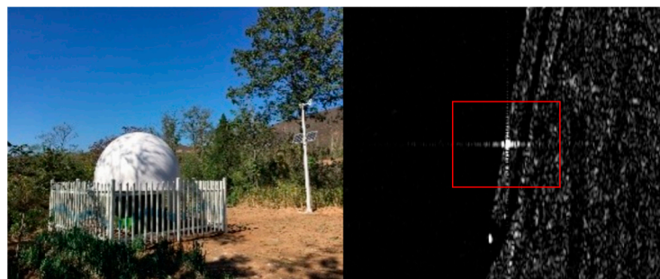
Figure 3. The appearance of CRs and the performance of CRs on SAR images
