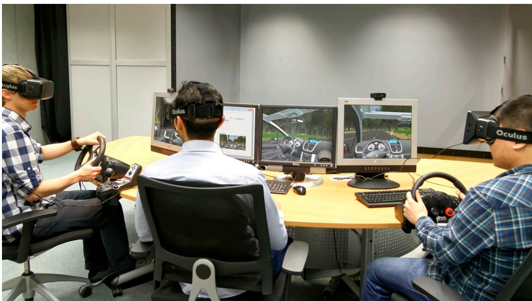
Figure 5. Prototypical implementation of the training platform with multiple head-mounted displays.
