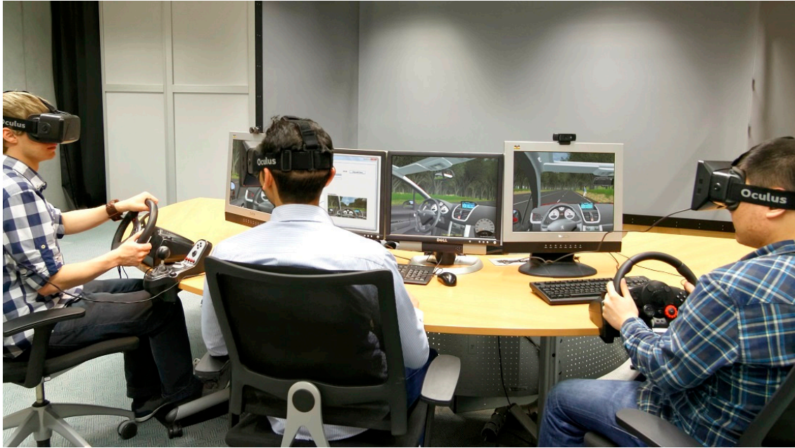
Figure 3. Prototypical implementation of ADAS training station with multiple head-mounted displays.
