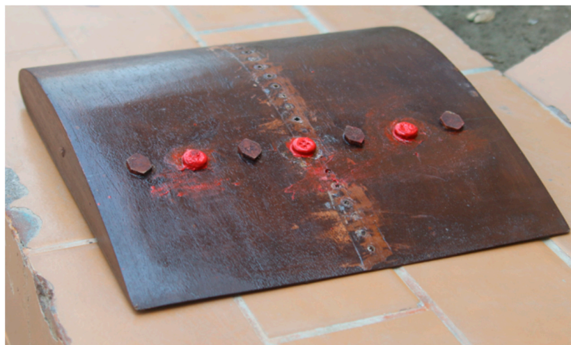
Fig.4.7. Prepared model with combination of hexagonal and circular dimples
