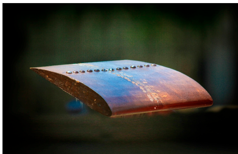
Fig.4.3. Prepared model with outward spherical dimples.
