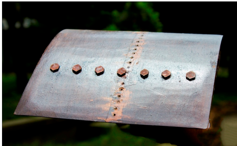
Fig.4.5. Prepared model with hexagonal dimples
