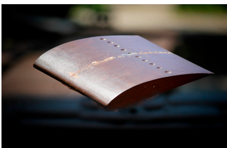
Fig.4.4. Prepared model with inward spherical dimples
