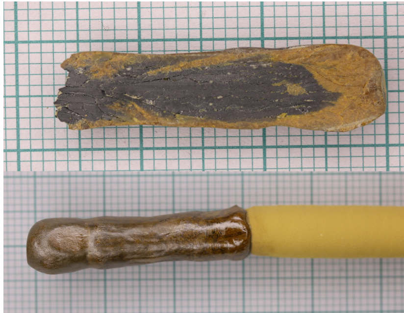
Figure 2. The result of growth 11 with 1.4% excess nickel oxide from stoichiometric. (a) The boule cut down the growth axis. There is a mixture of niobium-deficient \beta - \text{NiNb}_2\text{O}_6 (black) as well as polycrystalline columbite (yellow). (b) The as-grown boule.
