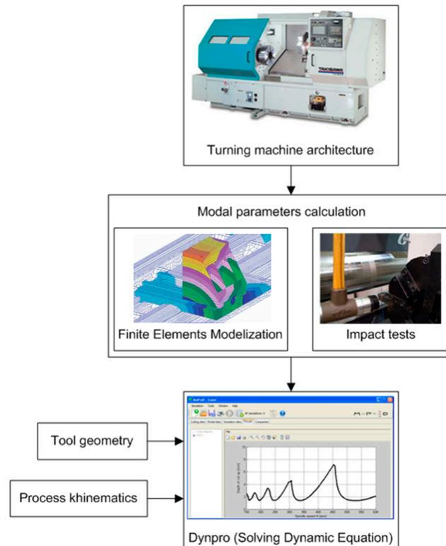
**Figure 10.** Experimental procedure for improved dynamic performance.
