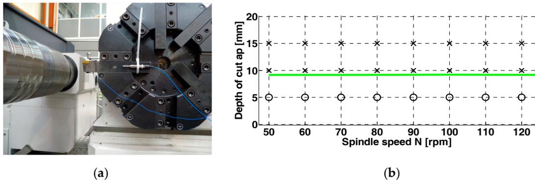
**Figure 13.** (a) Sound acceleration recording; (b) Stability lobes versus experimental points.
