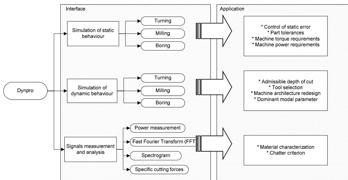
Figure 2. Functions and applications integrated in the approach.
