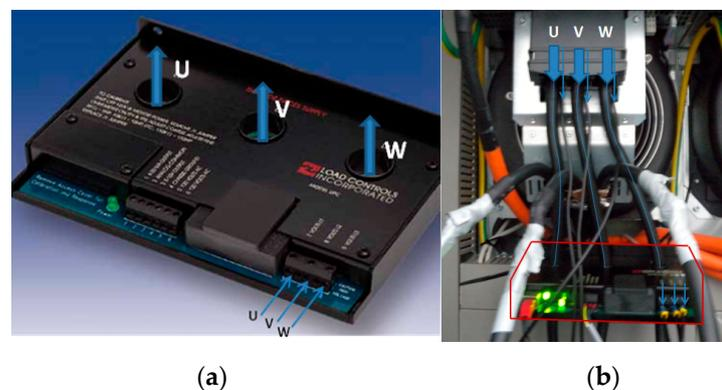
**Figure 11.** (a) Power sensor UPC-E; (b) Sensor installation on the plate motor.
