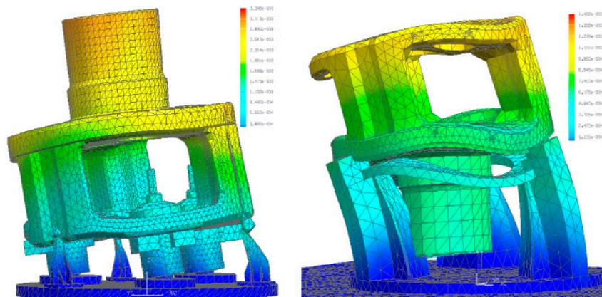
**Figure 9.** FEM model results for two fixture configurations.
