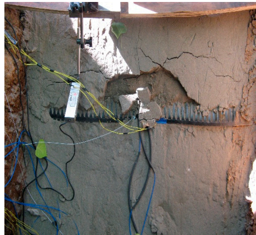
Figure 5. Crack development and damage of slope in the test.
