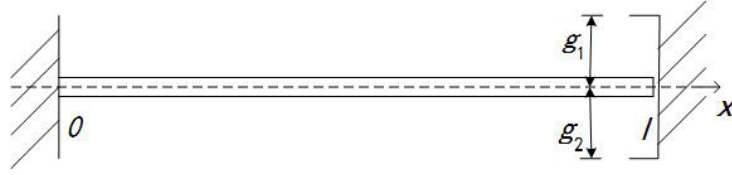
Figure 1: A thermoelastic Timoshenko beam and the tip at x = l with clearance g = g_1 + g_2 .
