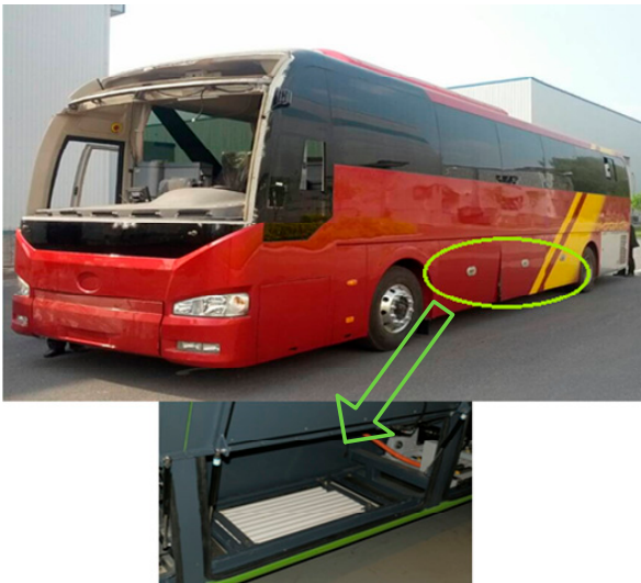
Figure 12.Electric bus and actual layout of heating pipes in battery box
