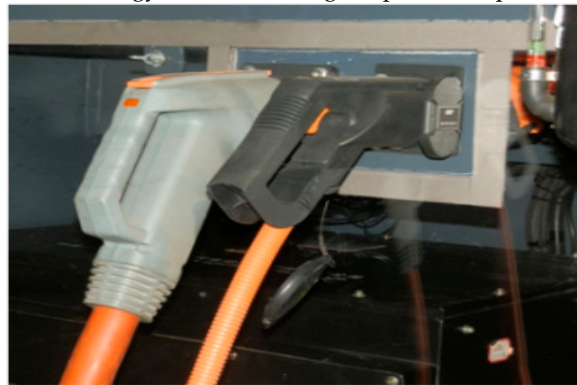
Figure 15. Charging plug (left) and heating plug (right)
