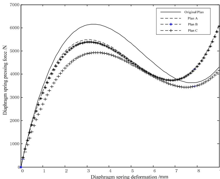
**Figure 5.** Characteristic curve of the diaphragm spring.
