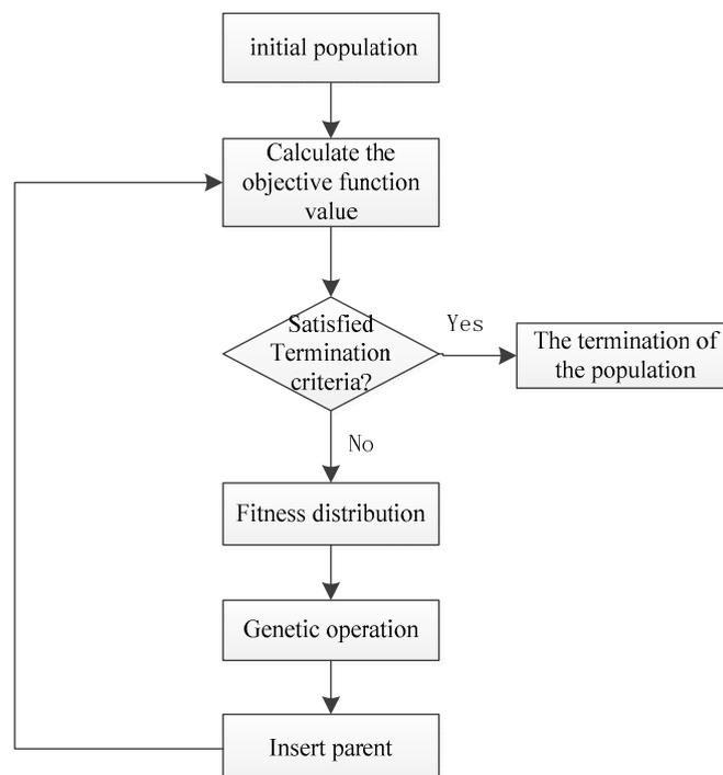
**Figure 3.** Non-dominated sorting genetic algorithm (NSGA)-II algorithm optimization process.
