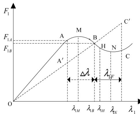
**Figure 1.** Characteristics of loading-deflection diaphragm spring.
