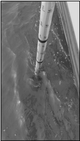
Figure 7. A pole mount system used for surface surveys (configuration-A). Here, a platform was equiped with MBS, DBS and a UWC systms on board of vessel.
