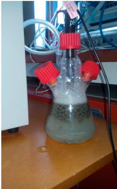
Figure 4: Reactor flask with sodium-alginate immobilized cells at exponential hydrogen production showing bead flocculation and excessive foam production at the neck of the flask
