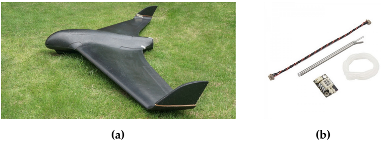
Figure 14. Sensor and UAV platform utilized in experiments. (a) UAV SkyWalker X8 with carbon fiber frame equipped with a 12x6 prop with 2x20g servomotor; (b) Digital airspeed sensor utilized in experiments which contains a 4525DO sensor which enables a resolution of 0.84Pa [28].
