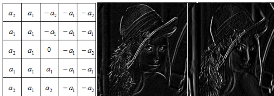
Figure 1. (1-a) Detection template; (1-b) Sobel operator detection effect; (1-c) FDMO operator detection effect
