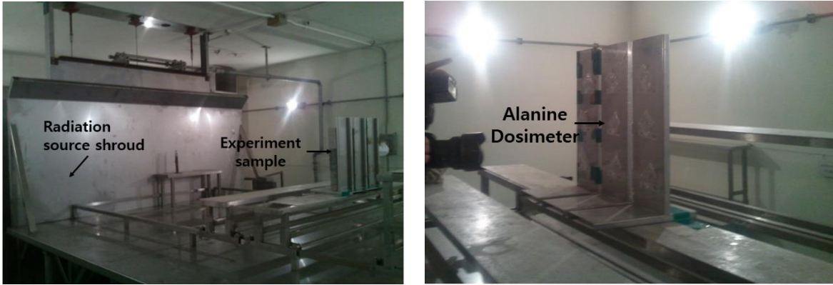
150 Figure 4. Experimental configuration for gamma-ray attenuation measurements
