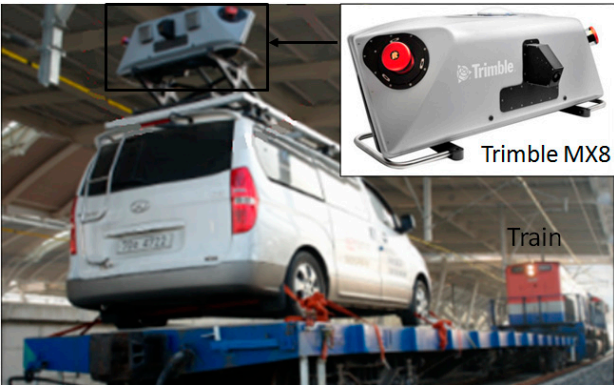
Figure 4. Trimble MX8 mounted on a train
