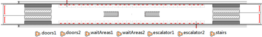
Figure 15. Simulation model of platform by Anylogic
