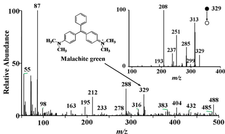
**Figure 2.** EESI-mass spectra of  $0.1 \text{ mg}\cdot\text{L}^{-1}$  malachite green obtained directly from water sample. The inset shows the  $\text{MS}/\text{MS}$  spectrum of malachite green ( $m/z$  329).
