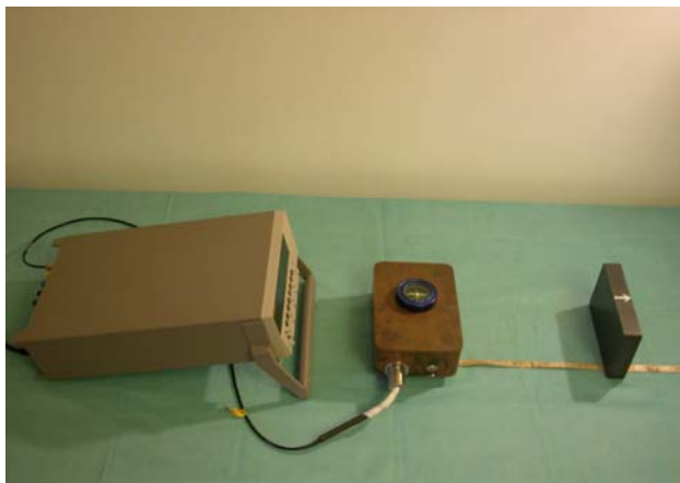
(a) a Keithley 6514, a shielding box and a magnet
