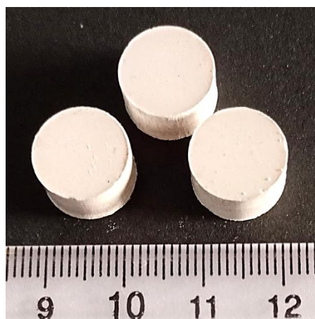
Figure 3. Photograph of three compacted pellets of \text{ZnS} at a pressure of 400 MPa. The numbers on the scale are in centimeters.
