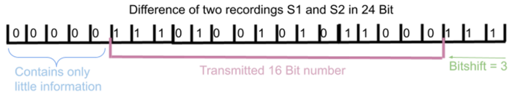
Figure 3. Bitshift Diagram: The calculated difference between S1 and S2 is a smaller value still represented in 24-bit. When the difference is small, the leading bits are zeros and carry no information. In contrast, when the difference is large, the initial bits contain significant information, while the later bits, representing very fine voltages, can be neglected.
