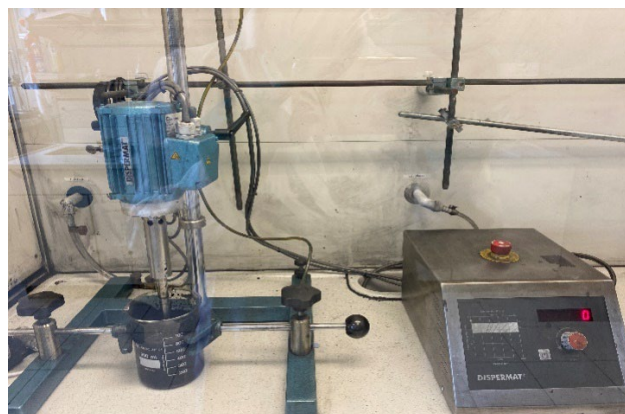
Figure 1. Screwed-on dissolver attached with the disk having D = 50 mm (Dispermat LC 30, VMA-Getzmann, Reichshof, Germany).
