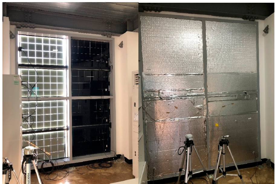
Figure 7. Interior view of the mock-up building with conventional and gray-colored BIPV systems installed.
