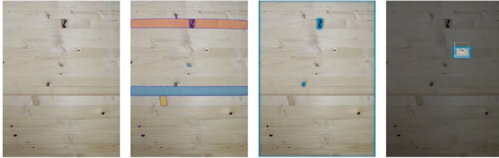
Figure 7. From the left - original image - mask prediction with “everything” function - mask prediction with bounding box corresponding to the size of the image - mask prediction with bounding box corresponding to a specific wood knot.
