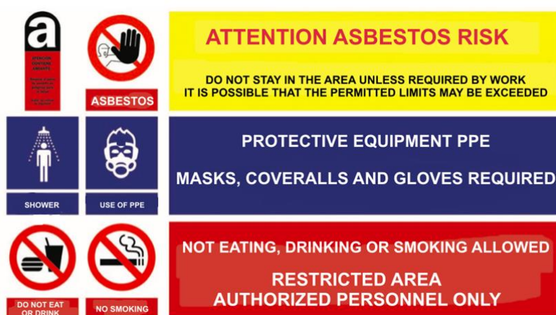
Figure 4. Examples of panels with representative warning signs used in asbestos-risk environments, modified from [46].
