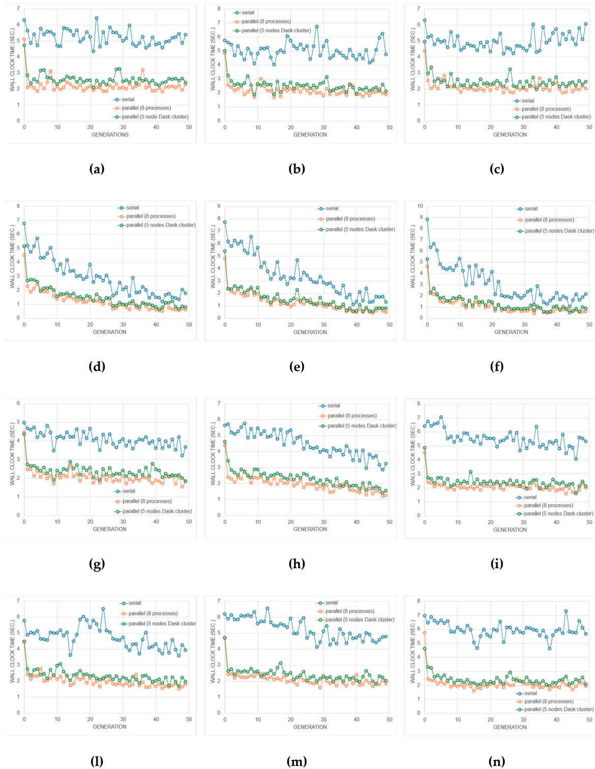
Figure 13. Evolution of wall-clock time per generation for different execution paradigms and SPICE-only optimization with NSGA-II, NSGA-III, and SPEA2, respectively, of the operational-amplifier topologies under test: (a-c) Miller-compensated differential amplifier; (d-f) Transistor-compensated differential amplifier; (g-i) folded-cascode op-amp; (l-n) Telescopic-cascode amplifier.
