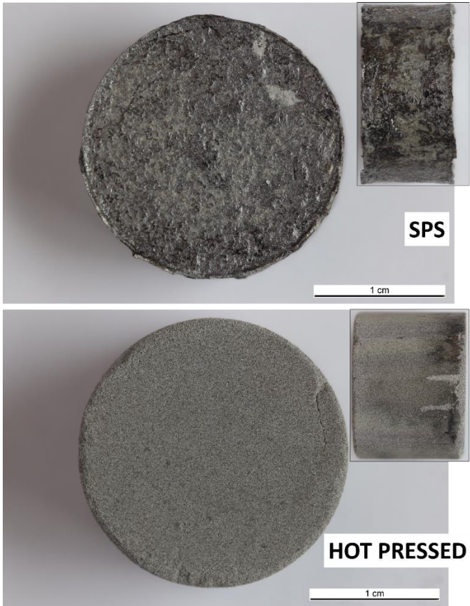
Figure 5. Optical images of the sintered sample by SPS and the pre-sintered pellet by hot pressing. The inset reveals the thickness of the sintered compacts.
