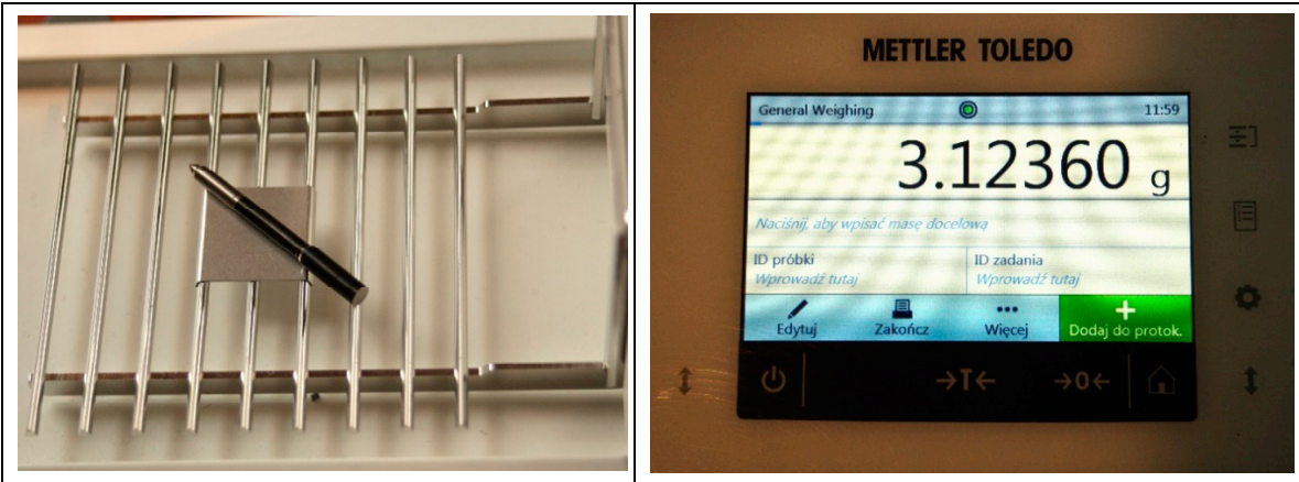
Figure 5. Measurement of the mass of the spray needle: a) placing the needle on the scale pan, b) result of the next weighing.
