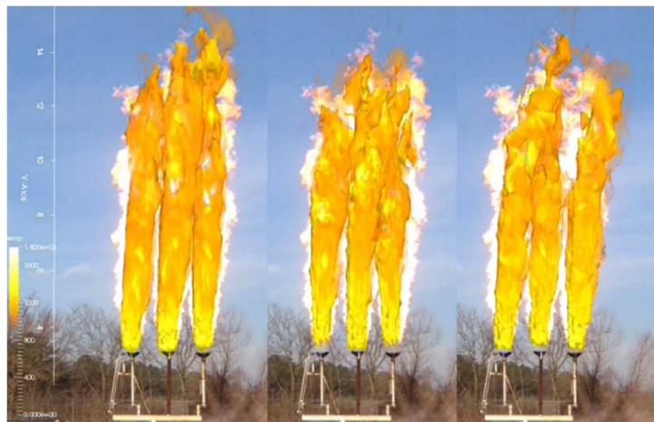
Figure 11. Comparison of Predicted and Measured Flame Shape for 3-Flare Test (sequential predicted images overlaid recorded flame image) [13].
