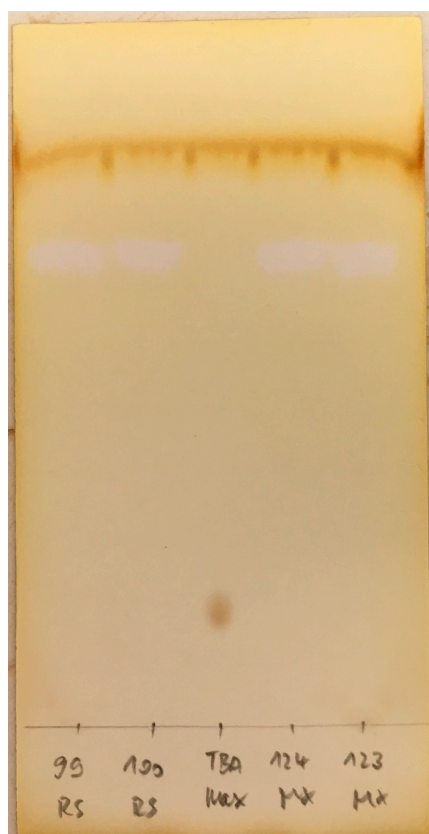
Figure 3: Iodine-stained TLC from the TBA test showing the reference solution 0.1 mg / ml in the middle and respective final solutions from TRACERlab MX (left) and mosaic-RS (right).
