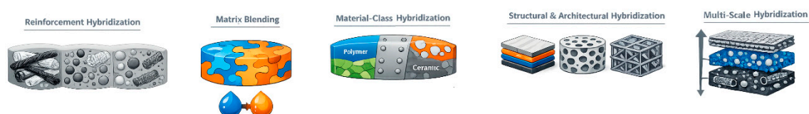
Figure 1. Schematic representation of hybridization classes in composite materials.
