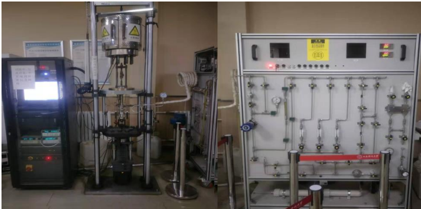
Figure 3. Slow Strain Rate Stress Corrosion Testing Machine.
